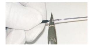
5. Cut temple tip to desired length with sharp blade, using trimmed metal piece as sizing guide
